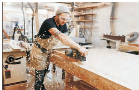
Carpenter working with an electric planer on a wooden plank. Photo via iStock.com/Monoliza21. [Used under license.]
